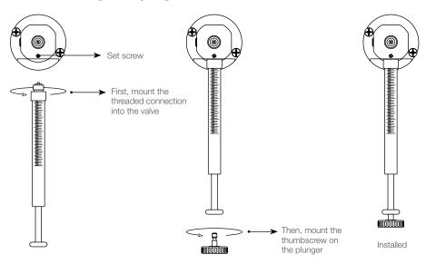
Important! Always tighten syringes so that they are fingertight. Syringes that are over- or under-tightened can cause problems with your Microlab 600.
