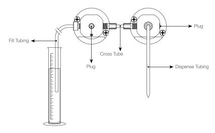
Figure 2-9 Dual Syringe Dispenser Valve and Tubing Assembly
