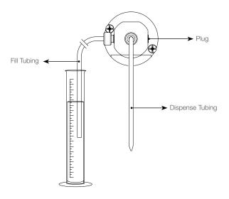
Figure 2-8 Dual Syringe Diluter Valve and Tubing Assembly
