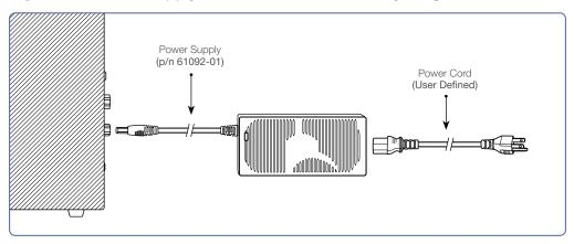
The Microlab 600 uses an external power supply like a computer laptop. The power supply is common to all Microlab 600 instruments and handles 110–220 VAC. When the Microlab 600 is purchased the correct power cord must be selected for the country where the instrument will be used.
