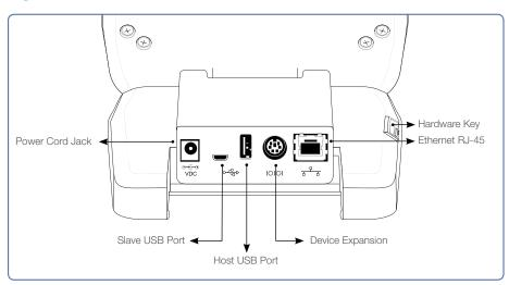
Figure 2-14 Rear View of the Controller
