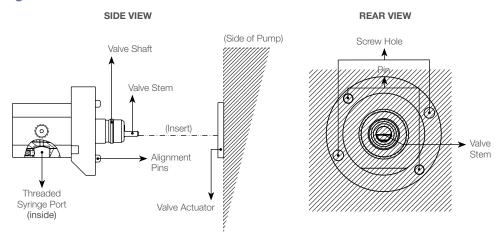
**Note:** The valve assembly will be installed on the Microlab 600 before it leaves Hamilton Company. For single syringe dispensers, the plug configuration will be as depicted in Figure 2-7. For dual syringe units, the valve assembly will be set as a diluter configuration.
