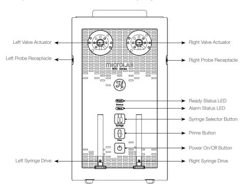
Figure 2-2 Front View of the Dual Syringe Drive Unit
