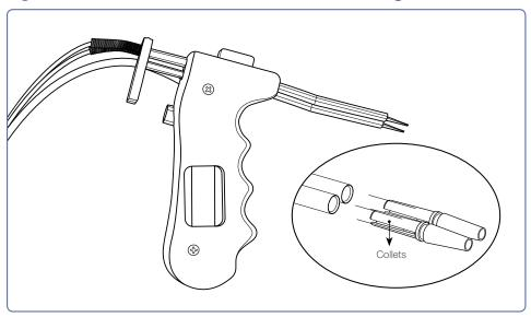
Note: The 18 gauge tubing requires the use of a tubing collet to hold the smaller tubing firmly. The tubing should be threaded through the probe to the desired length. Then the tubing collet should slide over the tubing and be slipped into the metal tip of the hand probe. As the collet is pressed into the metal tube it will grab on the tube to hold it firmly in place.
