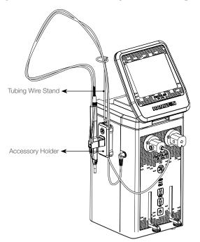
Figure 2-12 Final Assembly of the Tubing Management System
